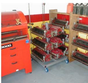
The lower set of reels lay flat on angle iron crossmembers with 1/4 inch keystock as stops to keep them from rolling. I started with 4 swivel casters but we changed 2 to fixed position ones and added a towbar similar to what a kids wagon would have. When we change out reels we take it our, swap the reels, roll it back in with the old reels ready for service. Saves some time and makes things easier to boot.
